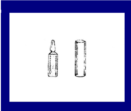
1. The ampoule is delivered in a plastic shield which prevents broken glass from the open ampoule from puncturing the gas release bag or from hurting one's hands.
