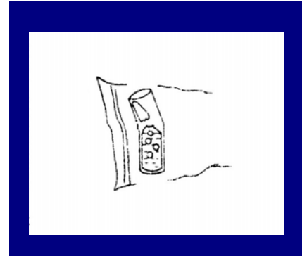
3. Grasp the ampoule through the bag and the protective shield and snap the top of the ampoule.
